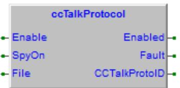
The **Fault** output is activated for a program loop in case of error.
