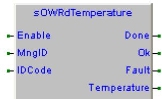
The **Fault** output is activated in case of error. Disabling **Enable** the **Done** and **Fault** outputs are reset, to execute a new reading the **Enable** input must be reactivated.
