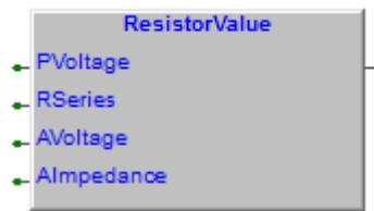
**PVoltage** (REAL) Supply voltage of the resistor divider (V)
