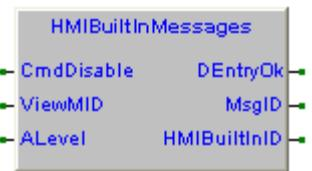
The **Alevel** parameter configures the access level to messages, setting the bits of the variable allows you to display only the messages that have the same bit defined in **Access Level**.
