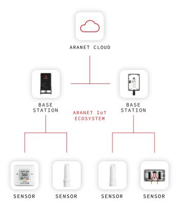
Aranet ecosystem is a simple and effective solution that can be integrated with 3rd party IT systems at two interconnection levels:
