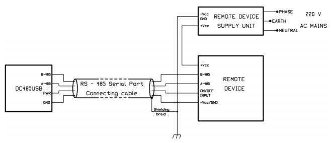
If the **PWR signal** is not used, the connecting cable may contains only 3 wires plus the shielding braid.
