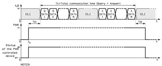
The TD1 and TD2 times may be unequal and depend on the characteristics of the controlled device.
