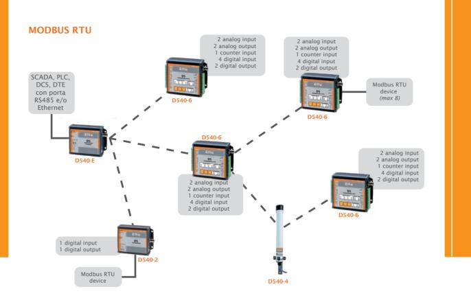
Network Modbus RTU point-multi-point with serial or Ethernet protocol (Modbus over TCP). Possibility to use routing tables to reach distant devices from the master unit and possibility of connecting additional nodes and devices Modbus RTU of third parties.
