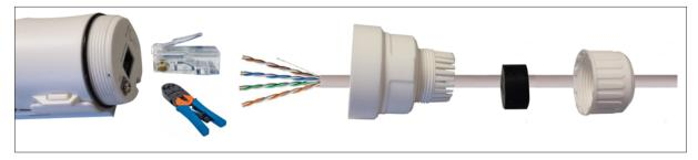
Use a Cat5e or Cat6 installation cable and thread it through the two plastic covers and the black rubber seal. Then use a crimp tool to affix an RJ45 plug to the cable.
