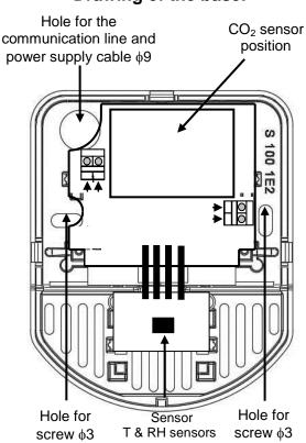
2. Put the drilling template on the expected location of the sensor or at a location where the supply cable is lead out from a wall and mark the position of drilling points with a diameter of 3 mm for the installation of the base and, if necessary, also a drilling point with a diameter of 9 mm for the power cable. The recommended working position of the sensor is defined in such a way that the round section of the box is oriented downwards – refer to "Base drawing".
