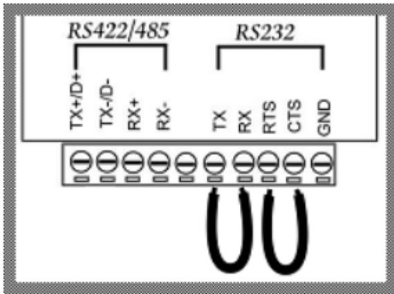
RS232 loop test wiring connection
