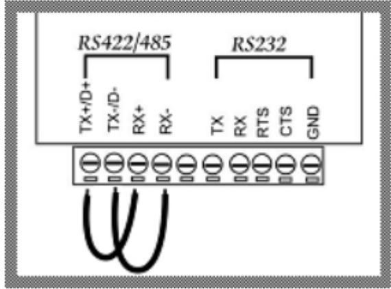
RS422 loop test wiring connection
