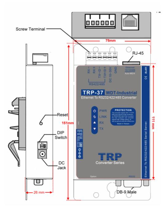
**Notice:** User can only choose either external DC-Jack or Screw terminal DC input. Do not use external DC-Jack and screw terminal DC input simultaneously.
