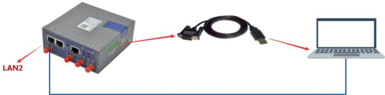
5.2 Open the PuTTY tool and keep spacebar press, then power on the router. Release the spacebar when the following appears.
