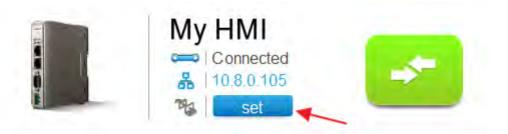
A window prompts for an IP address. Enter the IP address of the target PLC.
