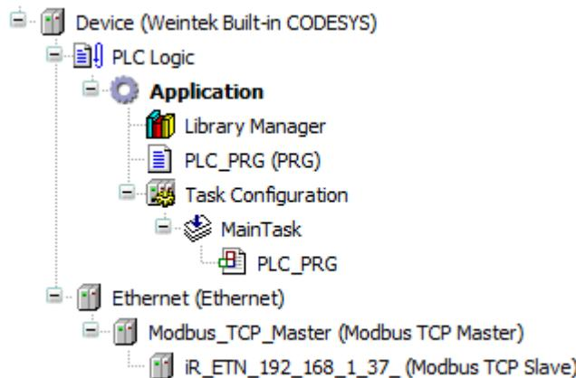
Read/Write channels and initial parameters are built.
